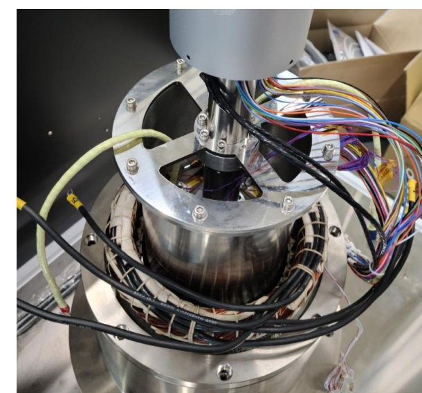
(a) Assembling the rotor and stator
