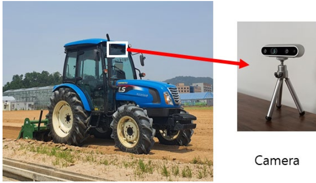
Fig. 2. RGB camera mounted on the front side of a tractor
