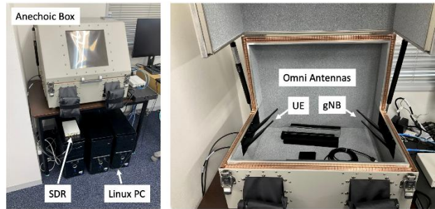
Fig.2. 5G Radio Access Network Verification System
