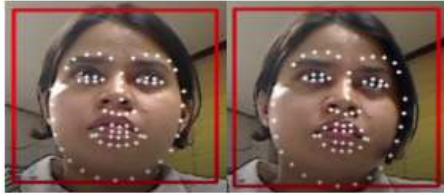
Figure 3: Facial keypoint detection with width multiplier = 1
