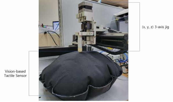
Fig. 6. Test environment for vision-based tactile sensor.
