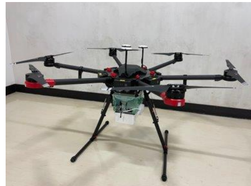
Figure 4: UAV with Millimeter Wave Device
