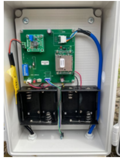
Fig. 3. Inside Monitoring Terminal
