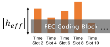
Fig. 2. Received signal at destination after applying phase dithering.
