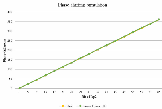
Fig. 11. Shifted phase according to the control bits
