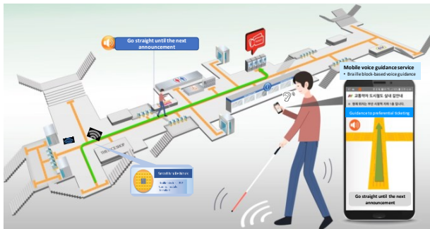
Fig. 1. Configuration of IoT-based route guidance technology for the visually impaired
