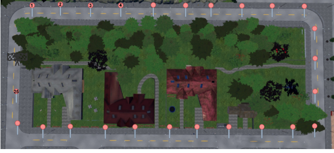
Fig. 1. Town02 Map in Carla environment [3] with a desired path that the vehicle should follow. The path is defined using waypoints represented on the map by blue bars with pink circles on them.
