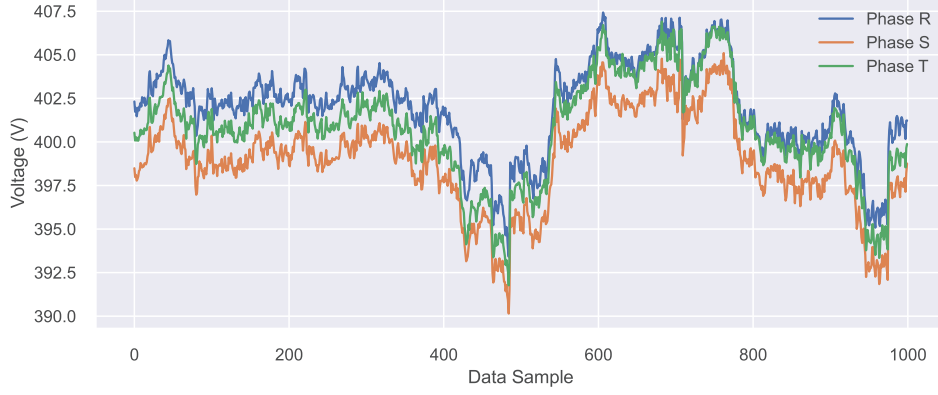
Fig. 2. Three-phase voltage profile of PCS.
