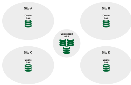
Figure 2. Phase 1: Normal situation: Centralised AAA is in sync with site AAAs.
