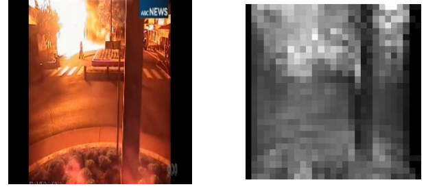
Fig. 3: The (a) original image of a fire captured by a surveillance camera and (b) the feature map that is processed by the first hidden layer at the UAV level.
