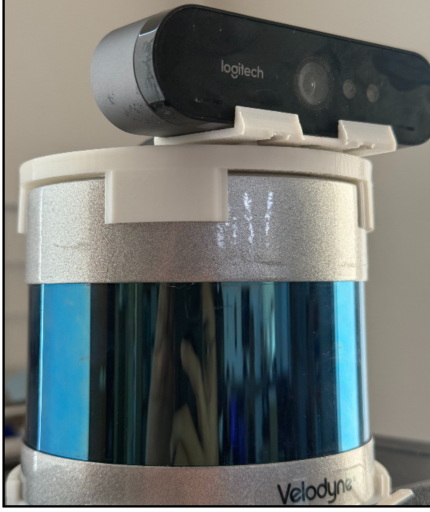
Fig. 2. Camera and LiDAR sensors mounting.
