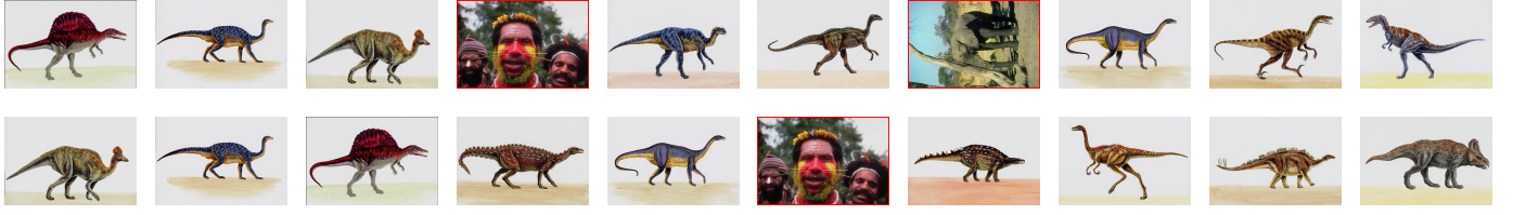
Fig. 3: Visual analysis of retrieving relevant images of “Dinosaur” class to a query image from the database using proposed CBIR scheme. Results for EfficientNet-B0 Block 7 is in the top row and for EfficientNet-B4 Block 7 is in the bottom row. The wrong retrieval results are surrounded in red box.
