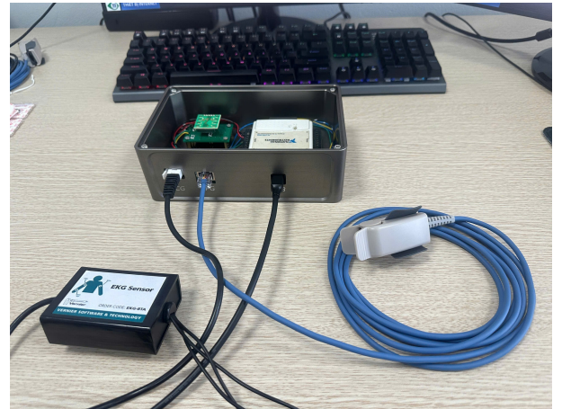
Fig. 6. Hardware architecture integrating non-contact radar sensing and reference contact sensors for multimodal physiological data acquisition in our Laboratory
