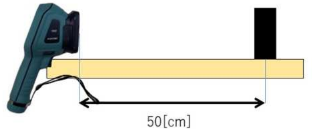
Figure 4. Experimental layout of the fan and microphone array. Measurements were taken at a distance of 50 cm.
