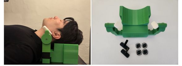
Fig. 4: Experimental Verification. The fabricated SafeDoze prototype applied to a healthy adult volunteer. The device elevates and stabilizes the mandible in an open-airway position, while the right panel shows the 3D-printed body and detachable components.
