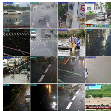
Fig. 6. Test result images of the flood classifier
