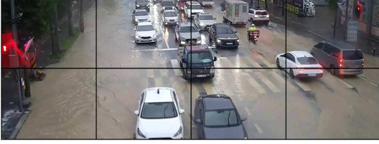
Fig. 7. Automatically configured 2 \times 4 grid over the bottom two-thirds ROI for cell-level inference
