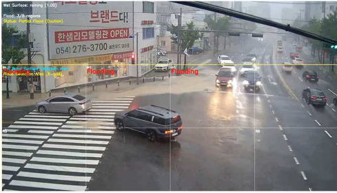
Fig. 8. Qualitative result on real flood footage: wetness classification of the roadway (Stage 1) followed by per-cell flood classification (Stage 2) across the 2 \times 4 grid.
