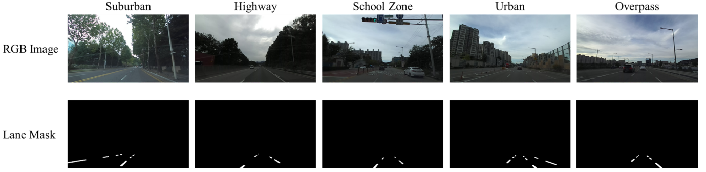
Fig. 2. Representative samples from the collected dataset. The dataset covers diverse driving scenarios including Suburban, Highway, School Zone, Urban, and Overpass to ensure environmental diversity. The top row displays the raw RGB images captured by the dashcam, and the bottom row shows the corresponding ground truth lane masks.
