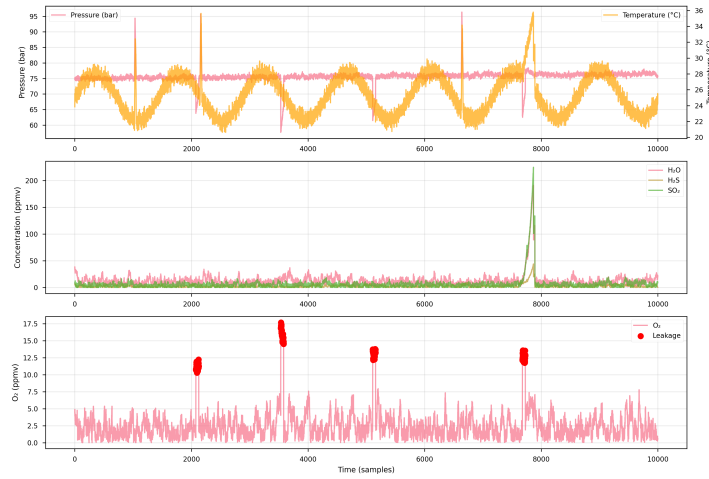
Fig. 6. Sensor time-series showing pressure, temperature, and impurity concentration dynamics.
