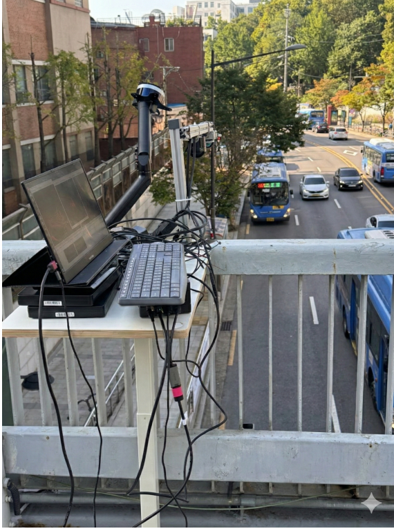
Fig. 7: Experimental environment: Configuration of RSU-mounted LiDARs installed on a pedestrian overpass near Hanyang University (Livox MID-360, RoboSense Airy, Velodyne VLP-16)
