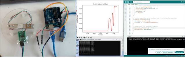
Fig. 3. Initial digital scale build and Real-time load cell monitoring.
