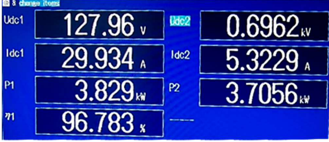
Fig. 4. Efficiency of a 3.5kW high-voltage current-type push-pull converter measured using a power analyzer
