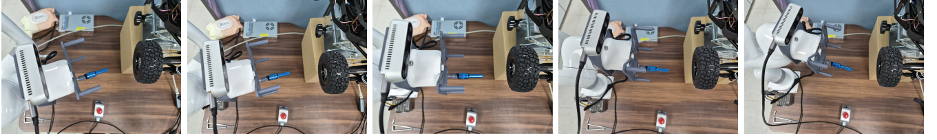
Fig. 5. Experimental setup for evaluating pose invariance under yaw variation: The robotic arm and the target wheel were positioned at -10^\circ , -5^\circ , 0^\circ , 5^\circ , and 10^\circ yaw (from left to right). Each configuration was tested with 20 independent trials.
