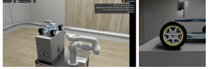
Fig. 7. Isaac Sim experimental environment (left) and recognition results in simulation (right)
