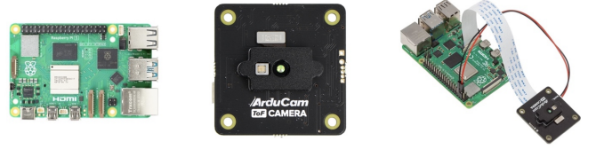
Fig. 2. The Arducam ToF camera connects via CSI to the Raspberry Pi Model 5, serving as the central computing resource for our Edge-IoT setup.
