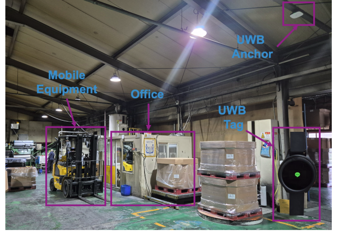
Fig. 4: Experimental setup for IISS operation, showing the UWB anchor, UWB tag, office, and mobile equipment (forklift). The driver’s line of sight is occluded by the office, creating a blind-spot scenario.
