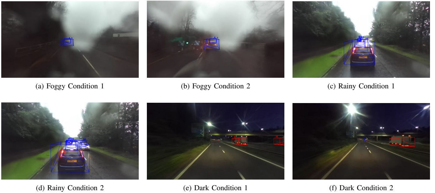
Fig. 3: Visualization of multi-object tracking results under various weather conditions like foggy, rainy, and dark. Each subfigure shows bounding boxes detected in challenging environmental scenarios: Insights from the RADIATE Dataset.
