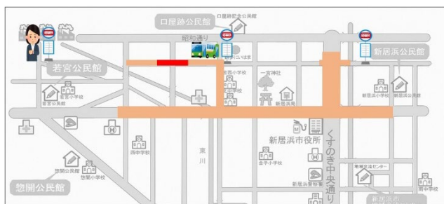
Fig. 5. Input image for machine learning. The congestion map, bus location, and speed are input for machine learning.
