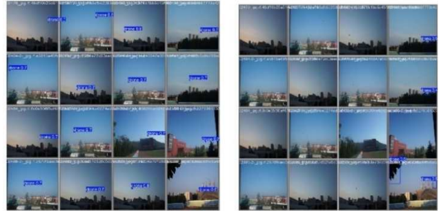
Fig. 7. Drone detection results using YOLOv11n on RGB images: model trained with RGB dataset (left four columns) versus model trained with infrared dataset (right four columns).
