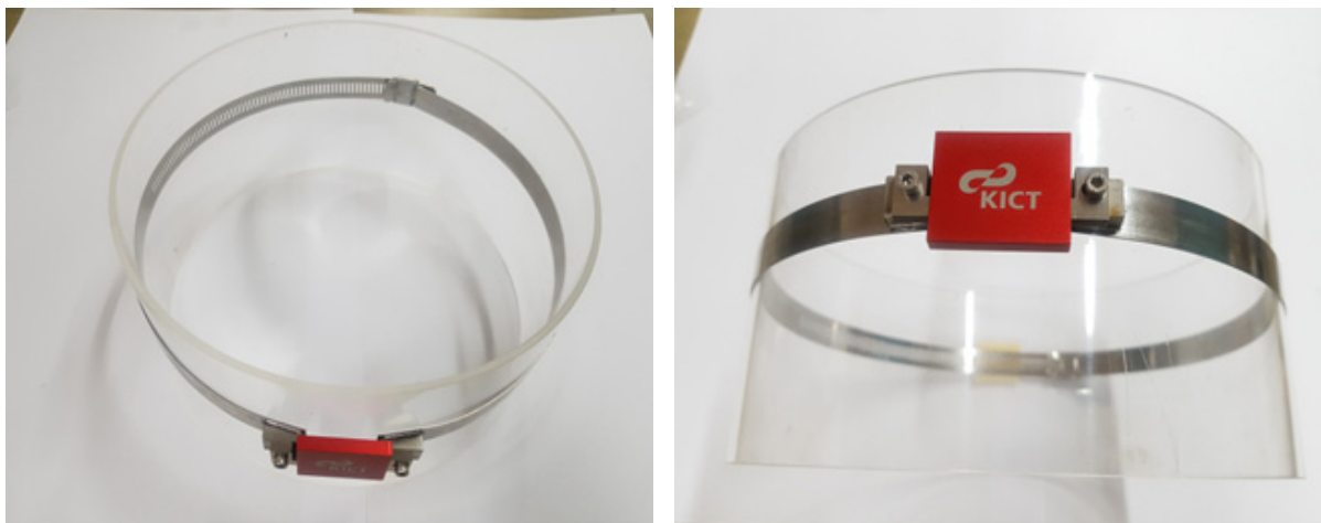
Fig. 1. The measurement system for the stability of chemical substance transport pipes as \phi 200
