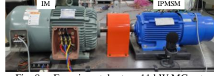
Fig. 8. Experimental setup; 11 kW MG-set.
